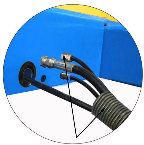
All the air hose and oil hose installed well as above manual are tied up and pass through Protecting plastic hose.
