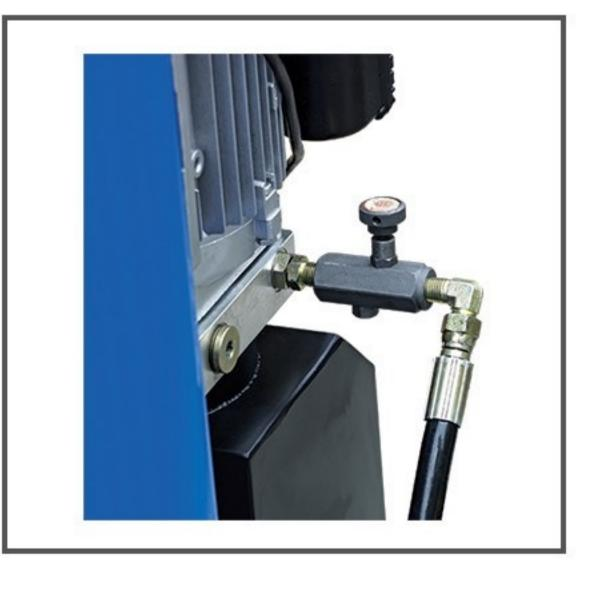
Even though all cylinders are flow restricted inside, we are adding the flow controlled valve to control the lowing speed for the heavy-duty line four post lifts model TFP14 and TFP14A
